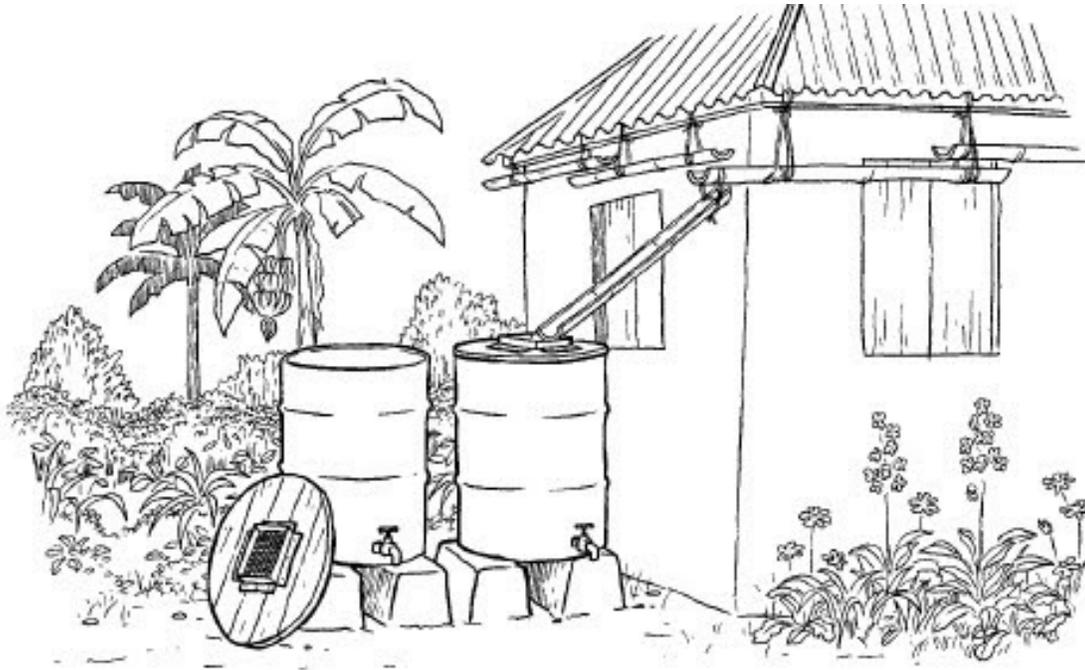
**Rain Water Collection for C.I. Roof**
